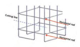
If you have to cut the grid before installation on the base, you must cut the vertical rod at mid distance between two horizontal rods as shown below.
