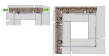
Take another stone and repeat the same process. Make sure you have a corner stone to finish the corner. Once installed, slide the stone along the horizontal axe to adjust the corner.
