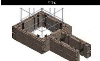
To integrate a wall into the column you must cut a veneer every two rows. The cut must be done at the middle of the dovetail.
