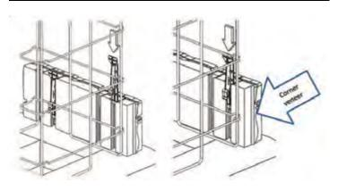
Take a veneer and slide the supplied connectors into the dovetails until they snap onto the horizontal rod of the grid.
