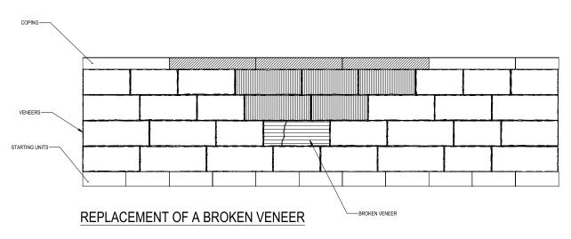
BEFORE REPLACING THE BROKEN VENEER, REMOVE ALL THE VENEERS AND COPINGS FROM TOP OF IT IN A "V" SHAPE. ONCE THE AGREGATES ARE DRAIN FROM THAT SPACE, REPLACE THE BROKEN VENEER AND PUT BACK THE OTHER VENEERS BEFORE REFILLING THE WALL.
