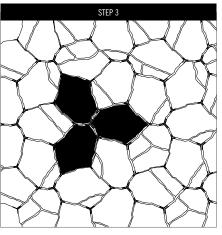
Complete the balance of the surface to be covered with single pavers.
