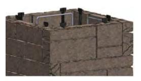
When you have reach the last row, cut the top portion of the connectors with pliers snippers or just by twisting the top portion with your hands.
