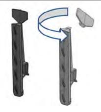
Apply glue on the top of the veneers before putting on the capping. IMPORTANT: The capping must lay on the veneers , not on the grid.
