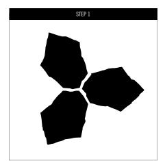
Begin by laying 3 pavers at the center of the surface to be covered.
