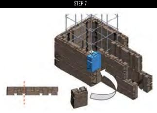
At the second row, cut a veneer (other than G format) at ther middle of the selected dovetail to fit with the space left.
